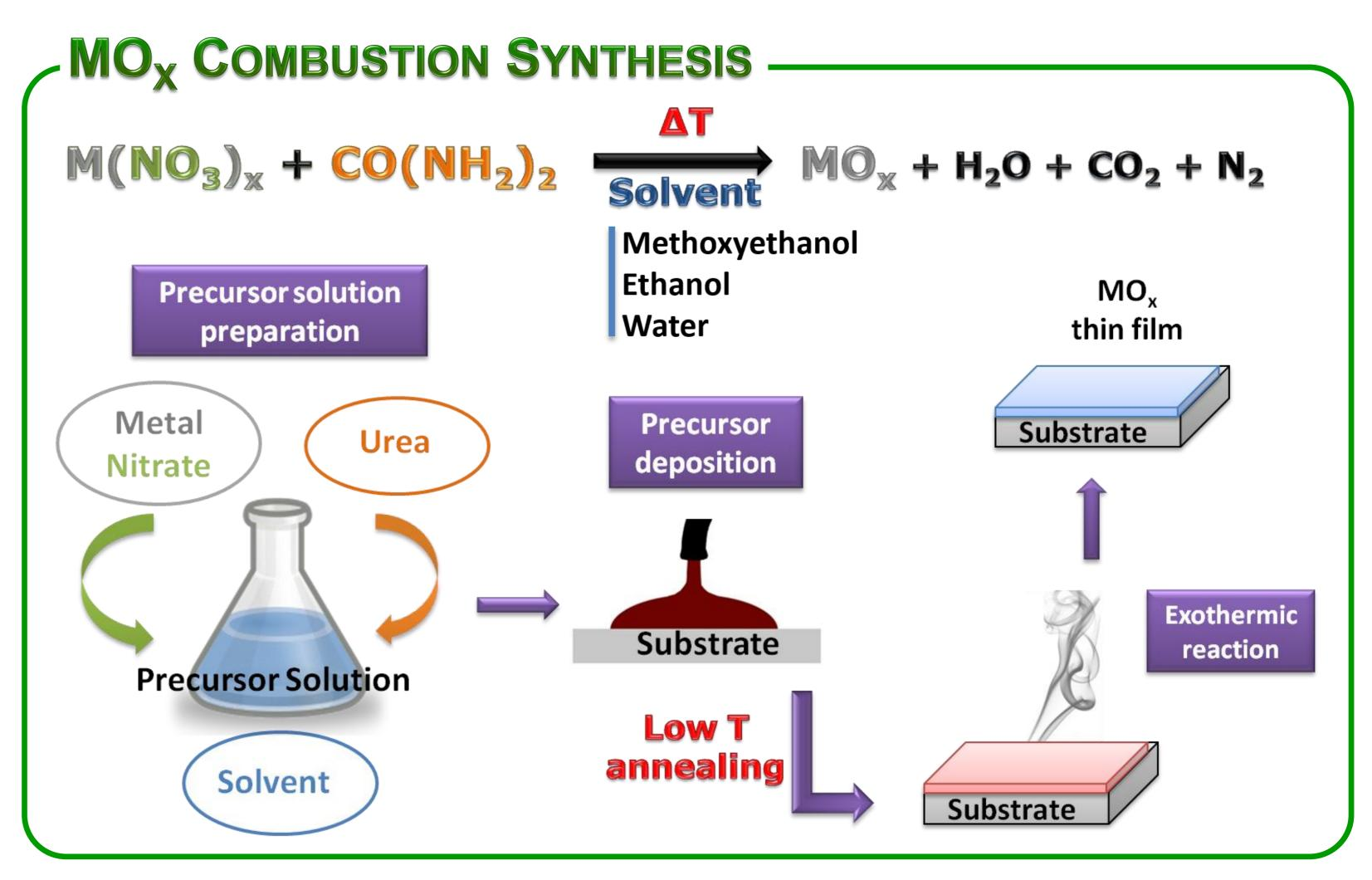
In this work the influence of several processing parameters; organic fuel, solvent and annealing temperature were studied. High performance devices are obtained and the results clearly show that solution combustion synthesis is becoming one of the most promising methods for low temperature flexible electronics. [1–4]
